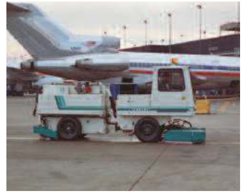
The 1550 efficiently picks up de-icing fluid from runways and covers 12 times the area of standard scrubbers without the need to empty and refill the solution tanks.
